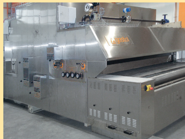
► inlet into oven with external humidifier
