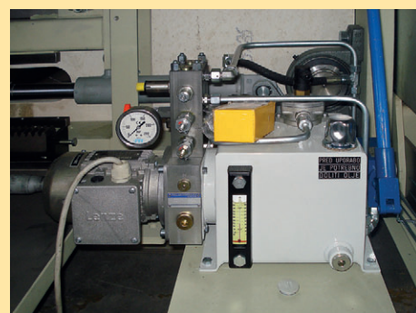
► hydraulic belt tensioning
